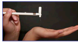
Each von Frey filament provides a constant force once it has buckled
