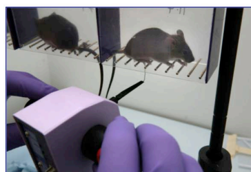
The MouseMet electronic von Frey has a 7gf range designed specifically for mice
